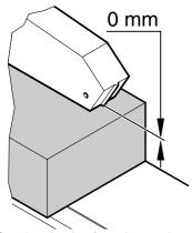
Set the depth of cut by turning the handwheel (68) on the chip case.
